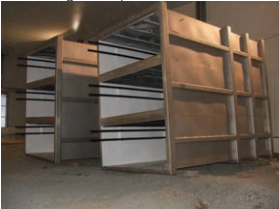
24 m 3 moving bed bioreactors for the small RAS 1 and 2 prior to installation.
