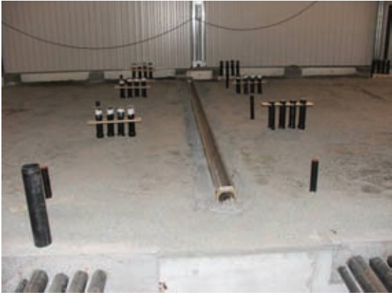
Outflow apparatus in the research hall. The arrangements permit a full range of options for water quality.
